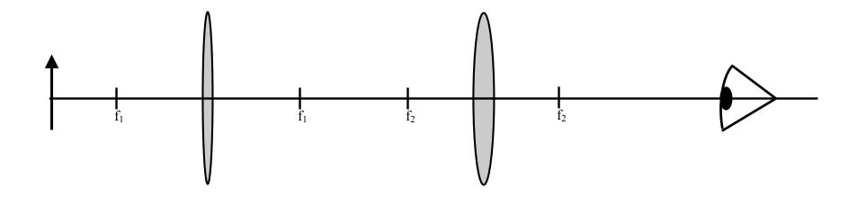
3. Locate the image of the object. Where might a lens system of this type be used?
