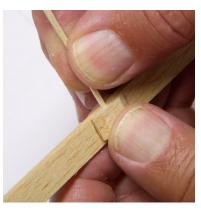
is re-assembled, the same relationship results. A second, equally important, outcome of using the socket and dowel connection is that the proper warps can be established for flying the airplane in a circular pattern. The word "warp" may sound like a bad thing for a wing and excessive warps are bad. The warps are actually given names like "Washin" and "Washout" because they help the airplane stay level in circular flight. See the section to about asymmetric construction and circular flight later.
