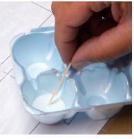
Use a scrap of the Styrofoam to transfer the cement from the can to the egg well so that the rim of the can stays clean. Mix in some water, about equal to the amount of cement and stir until completely mixed. Throw away the mixing scrap
