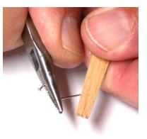
Make a second bend in the long leg at right angles away from the dip in the J.
