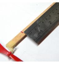
With a sharp razor blade cut a V-shaped grooves in the motor stick at the two marks from the top of the motor stick to its bottom. The groove should be less than 1 mm deep.
