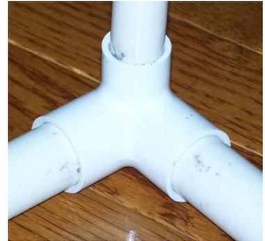
2. Use the  $\frac{7}{8}$ " drill bit to drill out the threads in the  $\frac{1}{2}$ " side of each elbow joint, as shown at right. Note the best way to stabilize the elbow during drilling is to insert  $\frac{1}{2}$ " pipe into the other 2 joints and clamp that pipe to your workbench:
