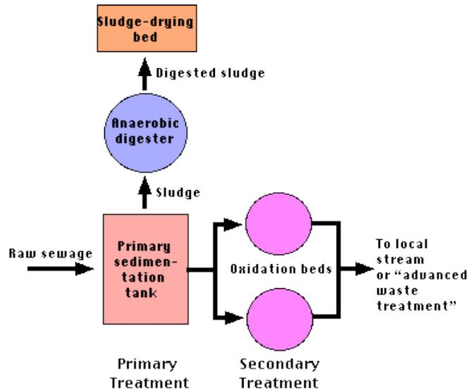
**Primary treatment** : The treatment step of sewage for physical removal of particles – large and small – from the sewage through filtration and sedimentation
