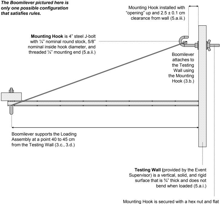
washer on the front side and a wing nut and flat washer on the back side of the Testing Wall (5.a.iii.)
