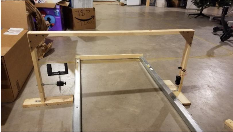
Photogate and laser rack. I glued magnets to the inside edges of the rack so they will attach to the rails and keep the rack in place.
