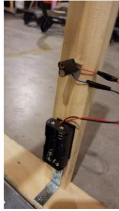
The photogate is mounted to a 1/4" threaded rod that goes through the rack and fastened with wing nuts inside and out. The photogate stem goes into part of a bracket sold by Vernier software (it has a 1/4" threaded rod in the middle of the bracket and made it easy to thread onto the 1/4" rod I used.)
