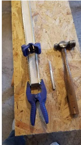
This shows the wood inserted into the metal stud. I clamped the stud tight, then used a punch to dimple the stud bottom, then drilled holes through the stud and the wood. Then I pounded nails into the bottom of the stud.
