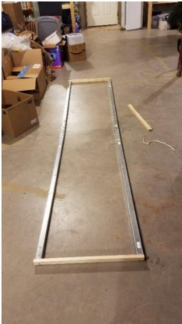
This picture shows the track opened up. The support board near the hinge has been removed. This fastens on with bolts and wing nuts through a hole drilled near the hinge. The support board and rope are lying next to the track. I used small steel studs instead of 2 x 4 metal studs. They are lighter and take up less space (from Home Depot).
