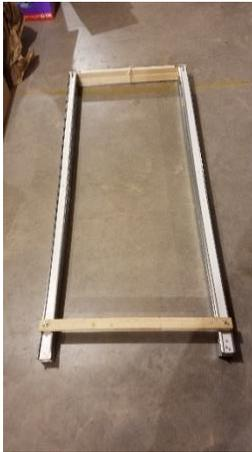
This version is hinged in the middle. This picture shows the track folded in half. I have fastened a piece of near the hinges for handling and travel. Otherwise the rails would move around damaging the track. A rope is tied around the boards that form the ends of the track.
