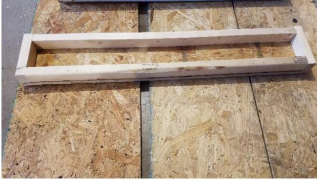
When folded, the edges of the track that will be in the middle (at the hinges) are very easy to damage. So I made a guard to fit over the track when folded. It is a rectangular box with a plywood side. This slips over the track when folded.
