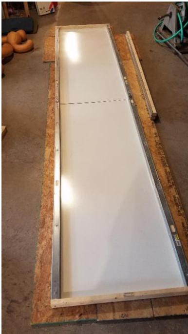
This is the track opened up. It is hinged in the middle (just like the above version). The plywood behind the track is just for working on it and is not part of the track.) The whiteboard is bolted and screwed to the rails. Because of the track dimensions, there will be a seam in the middle of the track. I will put mylar tape (used for fiberglass ducts in heating systems) on the seam.
