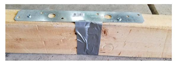
6. To transport the track, unscrew one side of each strap / steel angle to separate the pieces.
