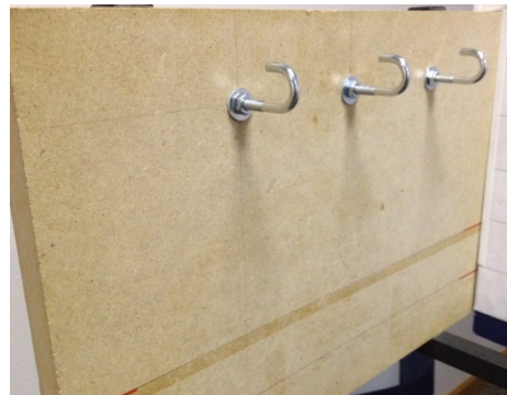
Figure B – Three hooks installed in wall for Division B. Only the center hook is installed for Division C.
