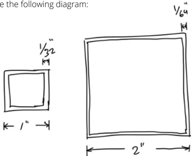
23. The two above square box girders have the cross-sections pictured above. Notice that they are different in both their outer dimension and wall thickness. Which of the below statements is true about the strength of the girders when loaded in compression axially down the length of the beam?
