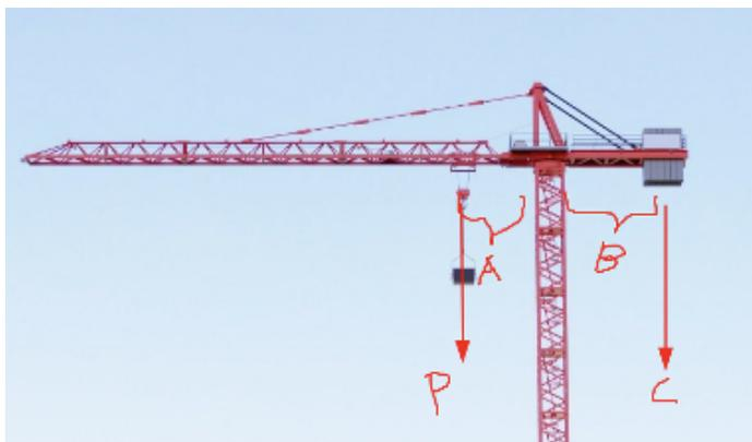
1. If  $P = 80,000$  lbs, and  $A = 12$  ft, how much should the counterweight weigh if the distance  $B$  was known to be 15 ft, so that the tower is only loaded in axial compression?
