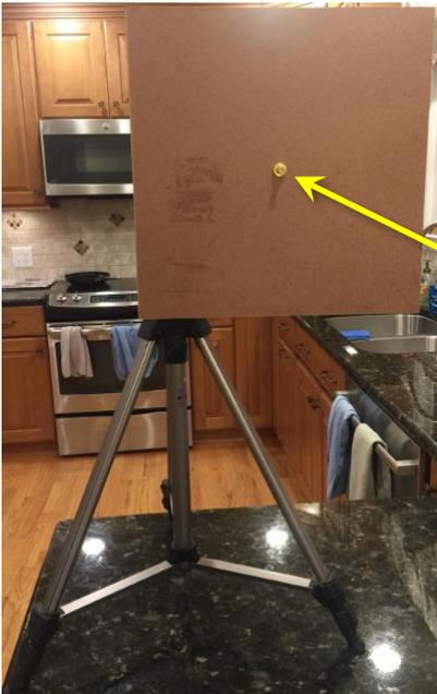
The left image shows the front of the backplane, where competitors' antennas will mount. Note the SMA-F connector in the center.
