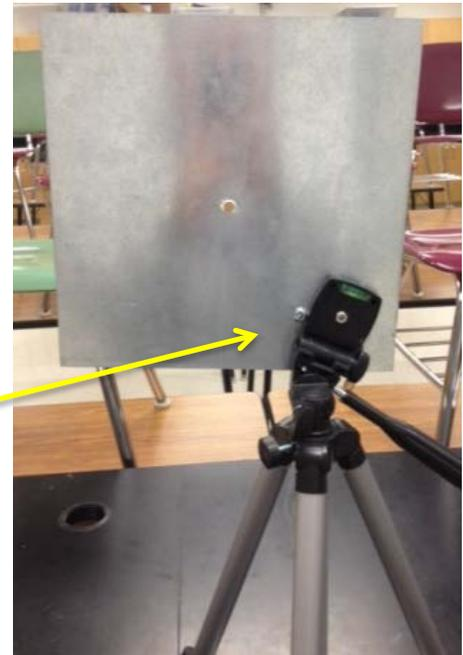
Unscrew the original antenna in the back of the WiFi router. You will not need this antenna for the transmitter but save it if you want to use the access point for the internet at a later date. Connect the RP-SMA male end of the antenna extension cable to the connector on the back of the router, and take the other cable end (SMA male) and connect to the bulkhead adapter mounted on the steel sheet.
