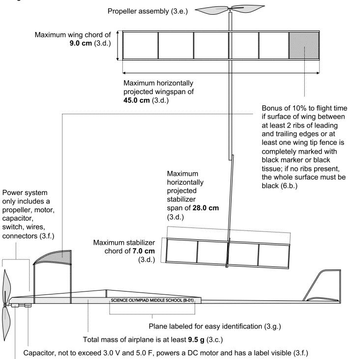
The motor directly drives the propeller without gearboxes (3.f.)
